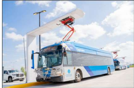
Bus and electric charging infrastructure
