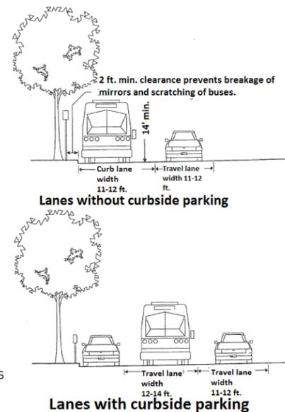
Note: lane widths narrower than 11 ft. will result in bus encroachment into adjacent lanes. Roadway Clearances for Buses (source: Tri-Met)
