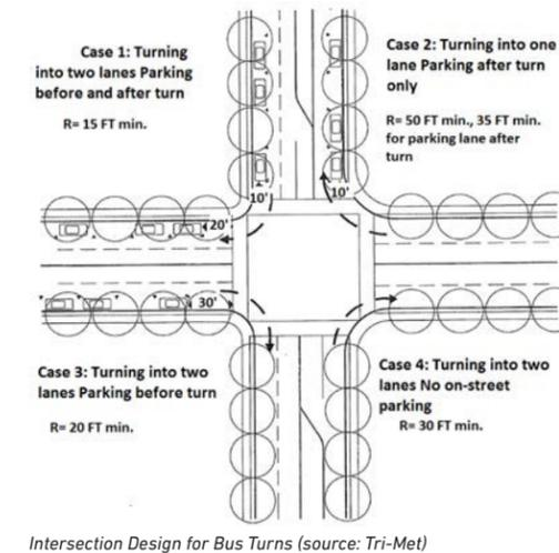
Intersection Design for Bus Turns (source: Tri-Met)
