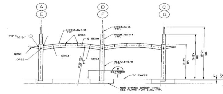
1 SIDE PLATFORM CANOPY ELEVATION SCALE: 1/4" = 1'-0"
