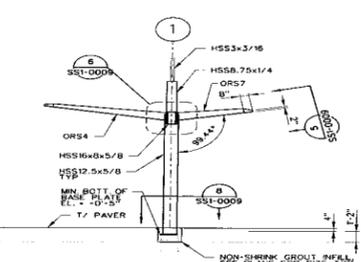
4 SIDE PLATFORM CANOPY ELEVATION SCALE: 1/4" = 1'-0"
