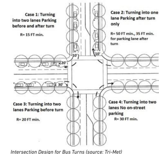
Intersection Design for Bus Turns (source: Tri-Met)
