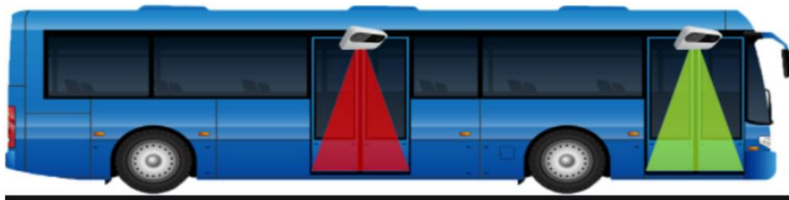
Automatic Passenger Counters (APC)
